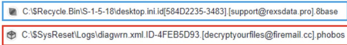
Figure 4: An 8Base file extension (top) compared to a Phobos file extension (bottom). (Source: VMWare)
